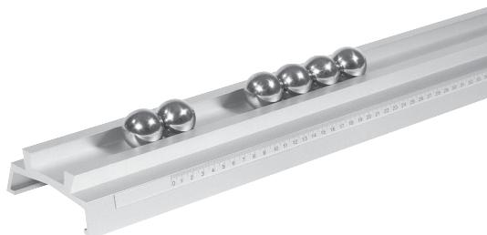
Steel balls suitable for experiments on elastic and inelastic collisions on a slide rail.
